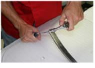
3. With vertical hardware removed, remove two horizontal straps.
