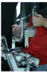
1. Remove existing shield from bike using quick detach mechanism.
